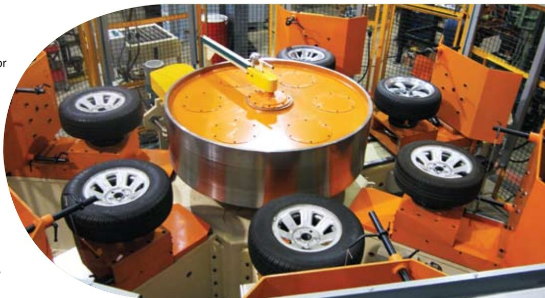
6 position Tyre Durability/ Endurance Machine (Overhead safety fencing removed for clarity)
