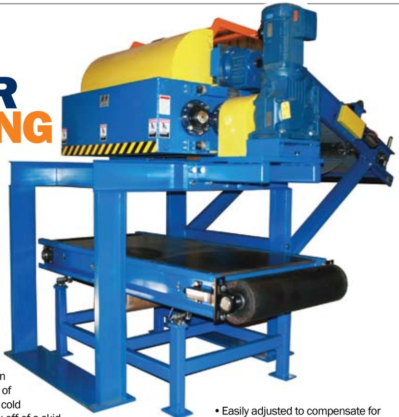
configuration pulls stacks of wig-wagged cold rubber stock off of a skid and cuts the width of the stock into pieces that drop onto a weigh conveyor. To reduce labor costs and provide for more accurate weighing, ASF varies the inlet speed of this feeder to automatically control and reduce piece size as the process approaches and then achieves the target weight.
