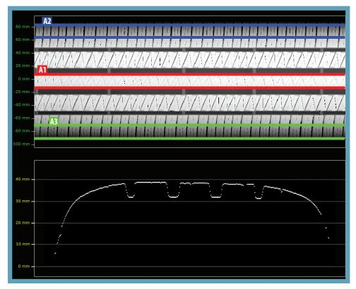
In addition to supporting a variety of 3D laser profile sensors from different manufacturers (e.g. LMI, Bytewise, Wenglor), the TSAS is also available with traditional 'spot lasers' which utilize our patented multi-path inspection software, and are significantly less expensive.
